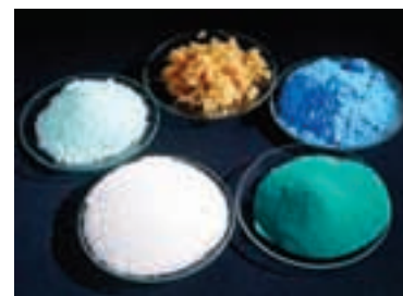
Figure 6.11 Clockwise from the lower left, the salts shown here are sodium chloride, iron(II) sulphate, iron(III) sulphate, copper(II) sulphate, and copper(II) carbonate.
