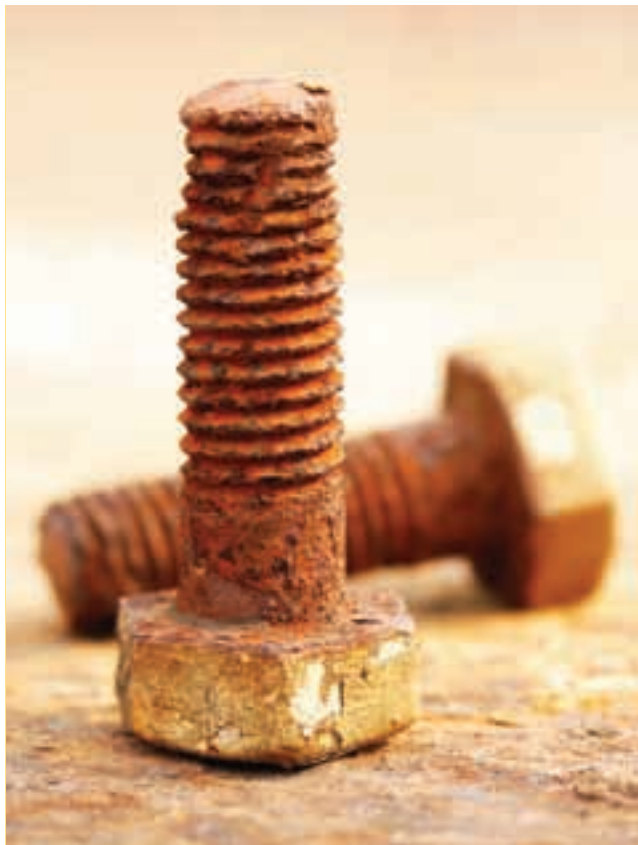
Figure 6.12 Rust contains iron(III) oxide, or \text{Fe}_2\text{O}_3 . Rust is produced when iron corrodes.
